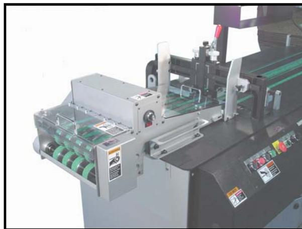
Convert the KR 215 into an inline transport using the KR 412 Shuttle By-Pass and use it inline with folders, tabbers, etc.
