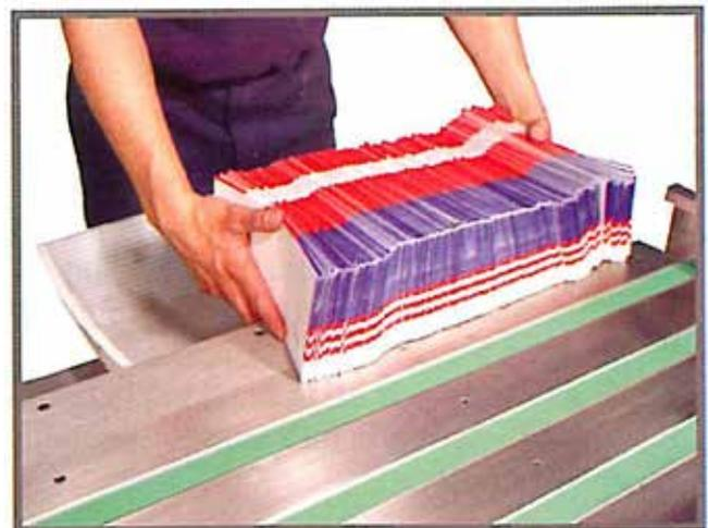
Fill trays in one motion by sliding bundles off the side of the conveyor.
